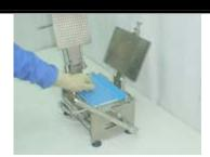
**19.** Place Caps Tray with Push Plate on Filler. Slide Push Plate off.
