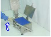
11. Release Cam Handle. This allows capsule bodies to drop so open ends are level with top surface of Filler.
