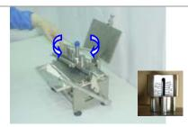
**17.** Turn Tamper Handle to compress powder & then reverse. Use Tamper Indicator for uniform compression between batches. Or, do a quick tamp as in photo 15.
